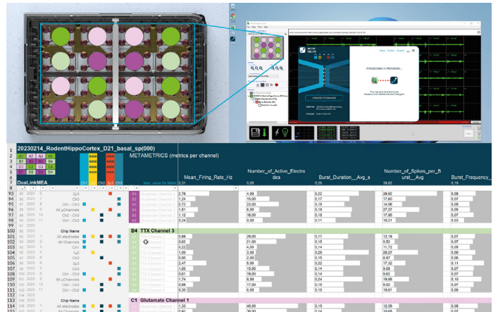
Figure 4: Screenshots of the UpLink software used to extract electrophysiological metrics. These metrics are organized in an Excel file per NeoBento™ with all compartment's configurations.
